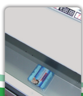
Thermal separator opening through an automatic closing above the drawer which avoids the release of cold and acts of intrusion detection.
