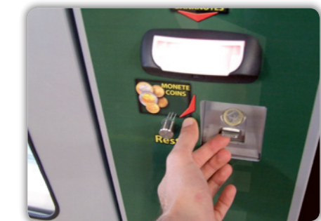
Mechanical reader that allows reading from 0.05 to 2 €
