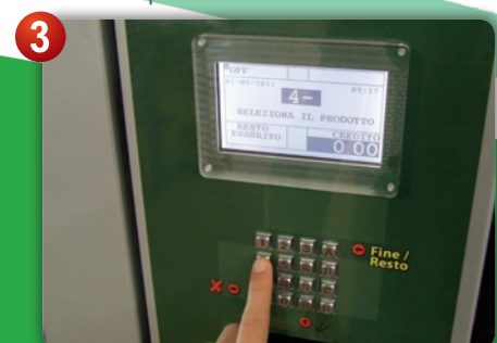
Large display that shows all the data relating to the sale and allows you to change all settings through a vandal-proof keypad with 16 keys.
